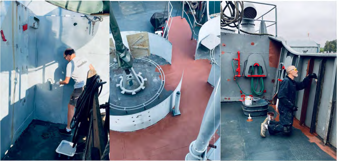
John is haze graying the bulkheads, primer on the gun deck, and touching up the new T-bar.
