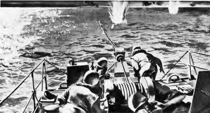
9 In a few minutes after starting the ramps, the crew puts all troops ashore and pulls off—under fire from 88 mm. batteries far inland. The boat backs out by pulling a cable attached to an anchor it had dropped coming in.
