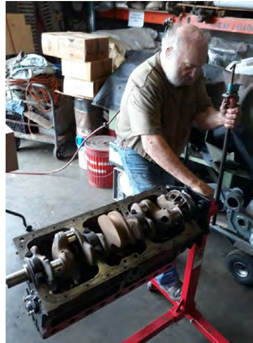
Steve Adams rebuilding the winch engine.
