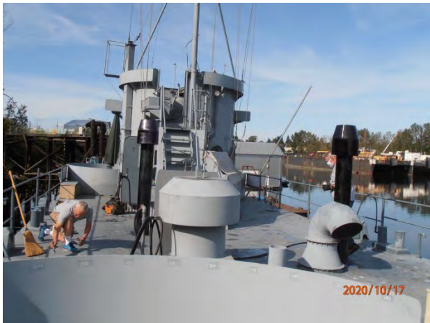
"Charlie Noble" vent stacks for the galley stove and boiler.
