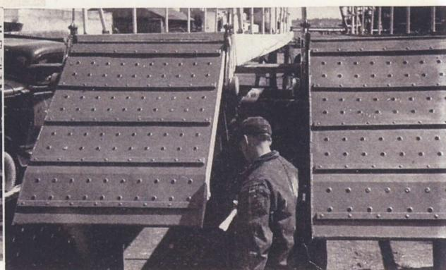
LANDING RAMPS are built separately also. This pair is ready to go aboard an otherwise completed LCI.
