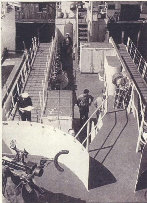
**DECK VIEW** showing both forward ramps safely secured in their sea-going position beside the inboard bulwarks.
