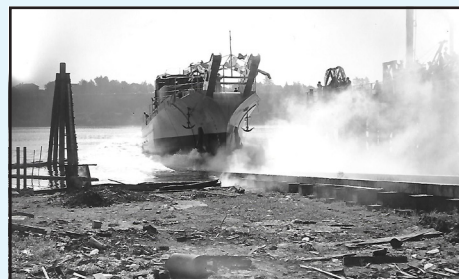
USS Buckeye is launched stern-first (back of the ship) down slipway into the Willamette.
