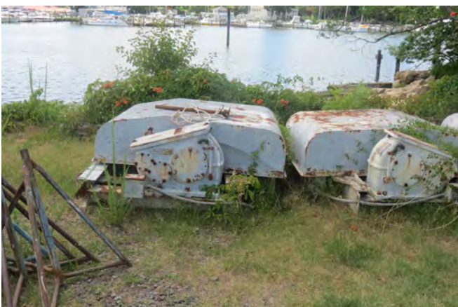
These unused Marine Railway Traction Motors could lift a ship on a cradle up a submerged ramp and out of the water.
