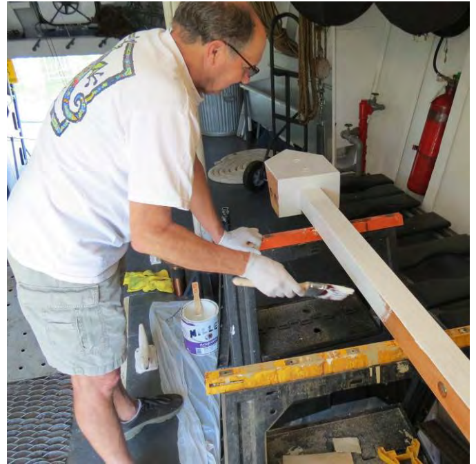
John paints the wooden Towing Spar (aka "Fog Buoy") that helps the ship maintain spacing in a convoy.
