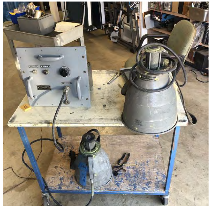
Amp shown connected to Megaphones for testing and microphone gain adjustment.
