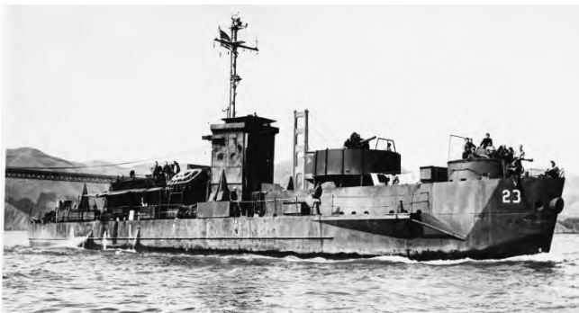
The LCI(G) 23 was one of the first four LCI conversions to gunboats.
