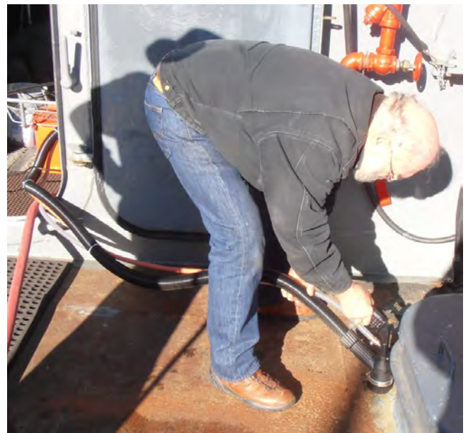
Steve with Vacuum blaster in action. Slow, but it works well on welds.
