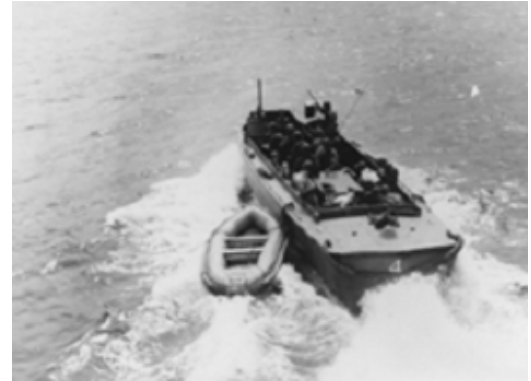
An underwater demolition team's LCP(R) leaves its fast transport (APD), towing a rubber boat, 3 July 1945. This shows the way the rubber boat is positioned for UDT swimmer discharge and the pickup below.
