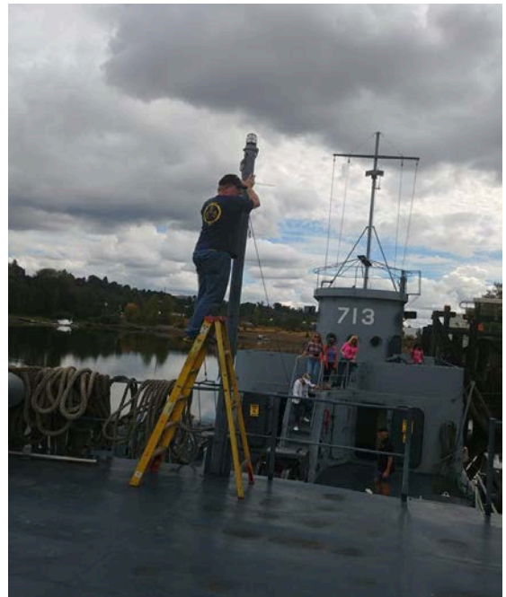
Di-pole antenna is completely re-worked and a new whip antenna for Ship's entertainment radio is added.
